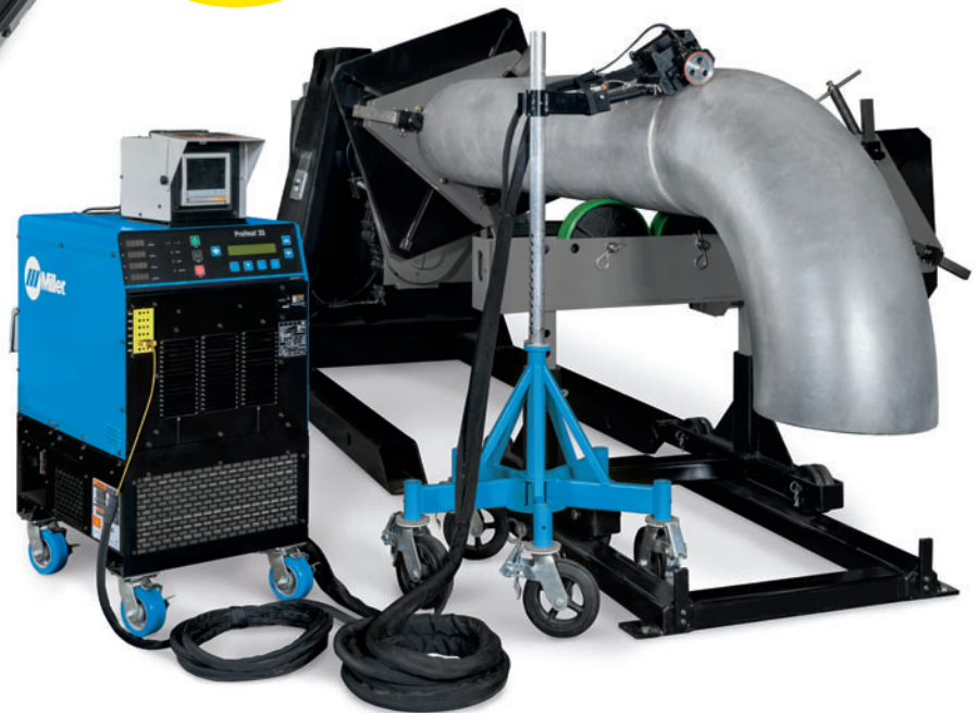
ProHeat 35 liquid-cooled system shown with complete Rolling Inductor setup. (Positioner and pipe stands sold separately.)
